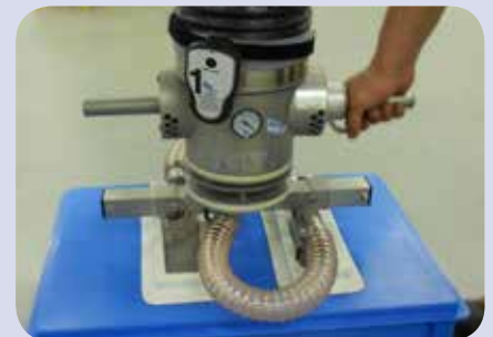
Operating knob in V2A with wireless transmitter
