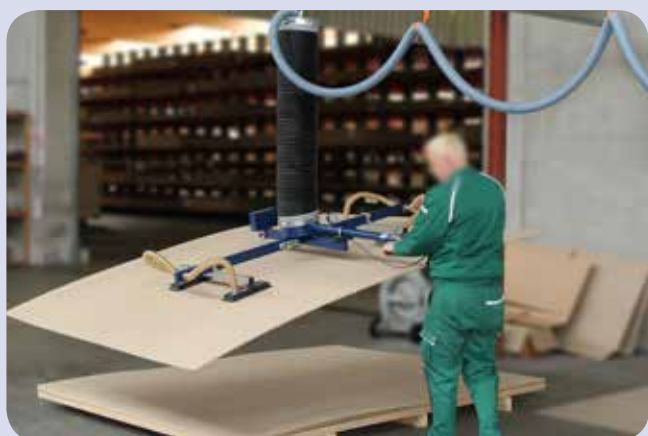
Lifting of porous wood panels with extended control handle
