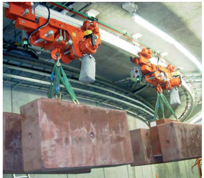
Electric Chain Hoist Type 29/06 EE ultralow headroom configuration with swivelling electric trolley capacity: 5 t
