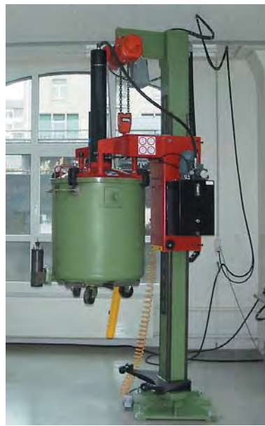
Electric Chain Hoist Type 66/04 AKS stationary used in the food industry
