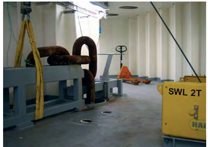
Electric Wire rope Winch Type 42/87 E capacity: 2 t used for service work on the platform's anchorage chains
